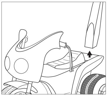
This vehicle features a removable handle so parents can "guide" young drivers. The handle is easy to remove when your child is ready. To remove the handle, use a Phillips screwdriver to loosen and remove the handle retainer screw (#12 x 1½") from the back of the vehicle and lift the handle. For storage, insert the screw into the hole in the back side of the handle. Store the handle and screw in a safe place for future use; the handle can be easily re-assembled to the vehicle at any time.
